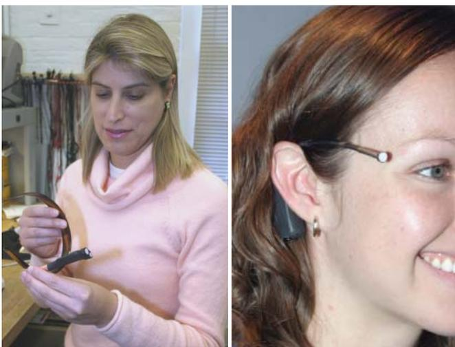
**Left:** LRC lighting scientist, Mariana Figueiro, PhD, demonstrates a prototype Daysimeter, a device used in field studies to measure circadian light entering the eye. **Right:** a recent version of the Daysimeter—smaller, lighter, and much easier to wear and use.
